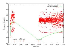
Figure 5: Throughput while A moving to EDGE2.
