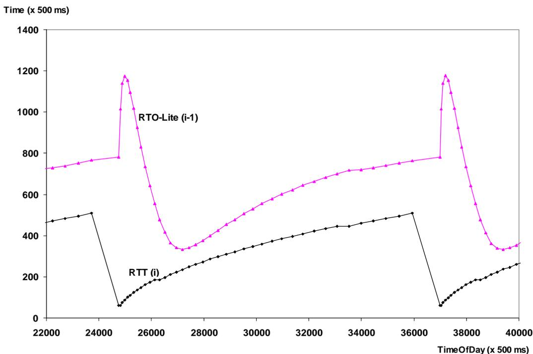
Figure 5-10:  $RTO_L$  when timing one segment per RTT.
