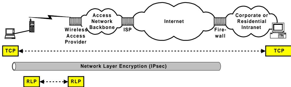
**Figure 2-18:** Getting secure access to an Intranet with an IPsec tunnel.
