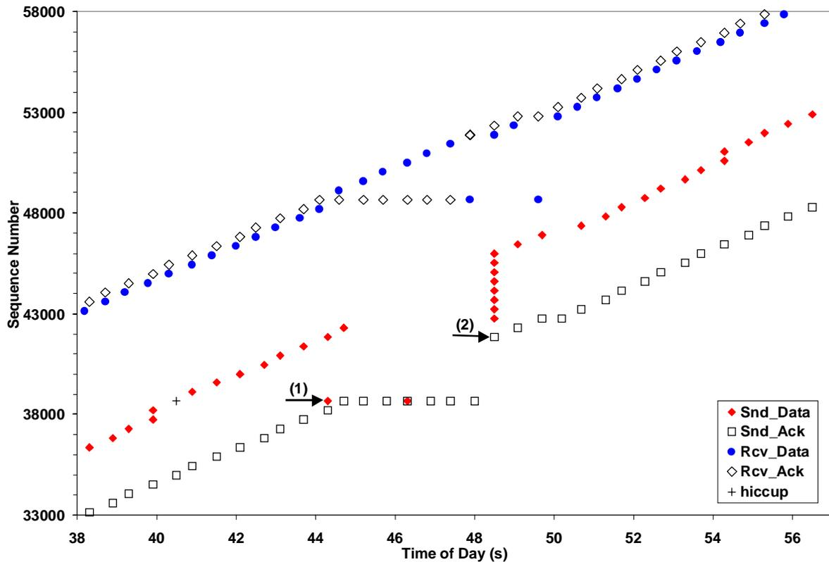
**Figure 5-6:** Response after a spurious fast retransmit.
