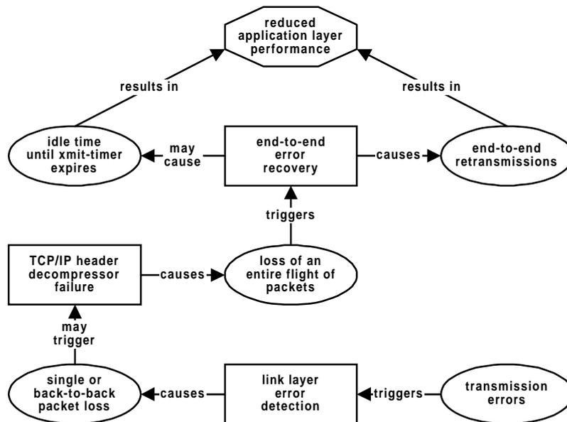
**Figure 2-15:** Cross-layer interaction leading to the failure of TCP/IP header compression.
