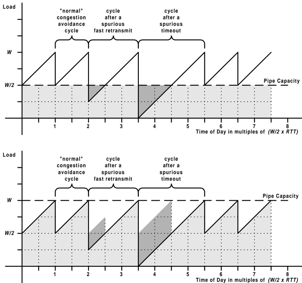
Figure 5-7: Approximating the performance loss.
