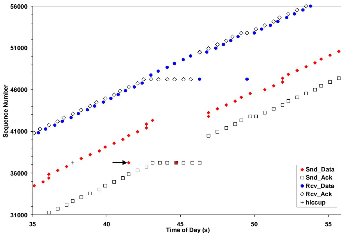
Figure 5-4: The effect of packet re-ordering.
