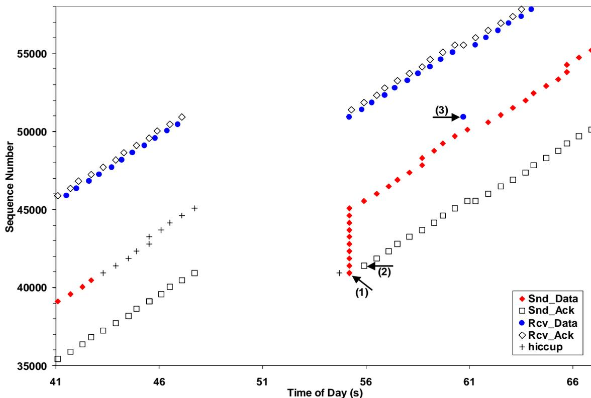
Figure 5-5: Response after spurious timeout.
