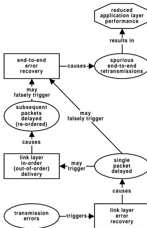
**Figure 2-14:** Cross-layer interaction leading to competing error recovery.
