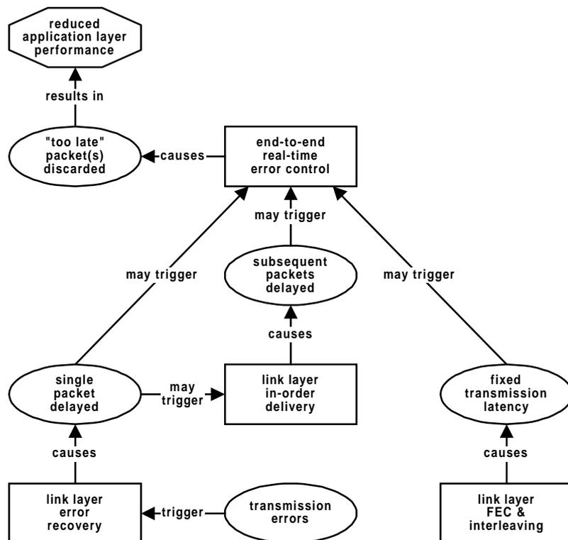
**Figure 2-12:** Cross-layer interaction caused by overly strong link layer error control.
